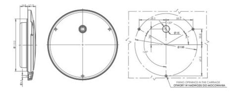
The lamp is assembled inside with the use of three screws hidden in a chrome-plated ring with a diameter of 152 mm. It is encased in an opening with a diameter of 113mm with only approx. 18mm protruding from the surface to which it is assembled.
